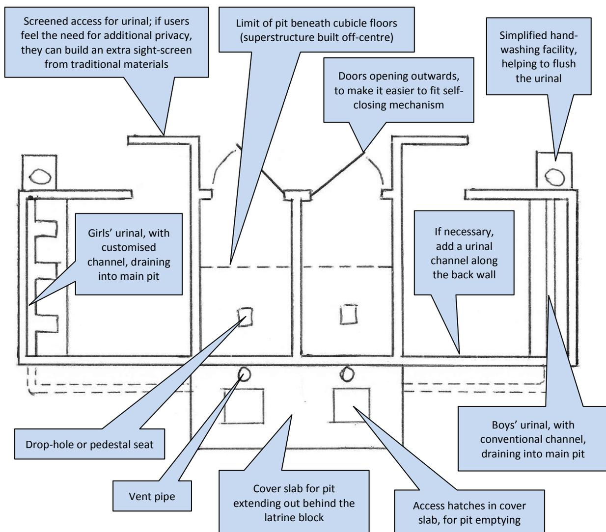
This layout is suitable for a primary school or as the staff sanitation block in a large secondary school. For other situations, the design can be treated as modular, with components multiplied, expanded or separated as necessary.
