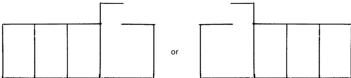
The number of cubicles in these blocks can, of course, be varied according to the size of the school. In addition, the length of the urinal can be increased for larger numbers of users:
