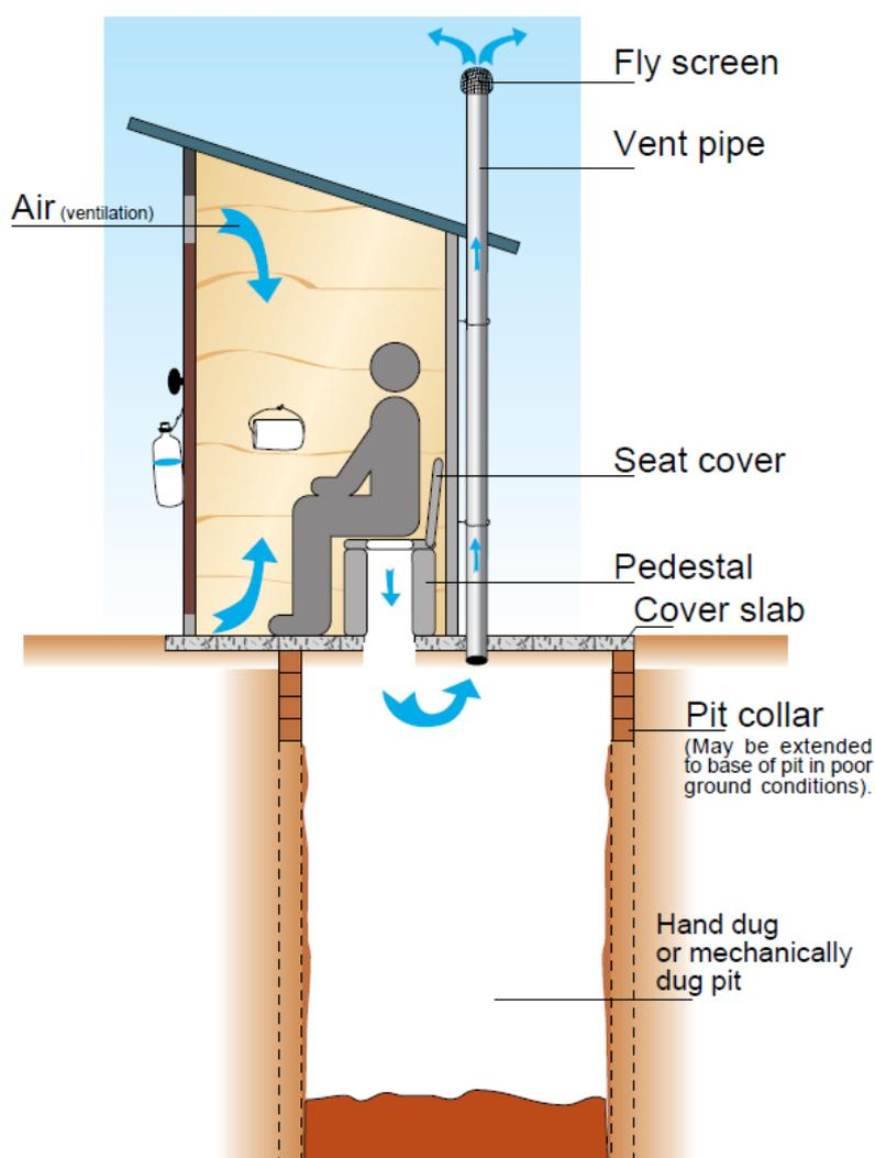
The pit eventually fills up, as not all solids are broken down. It is then either emptied, or the pit is sealed and abandoned and a new latrine constructed elsewhere. Separate hand-washing facilities are required.
